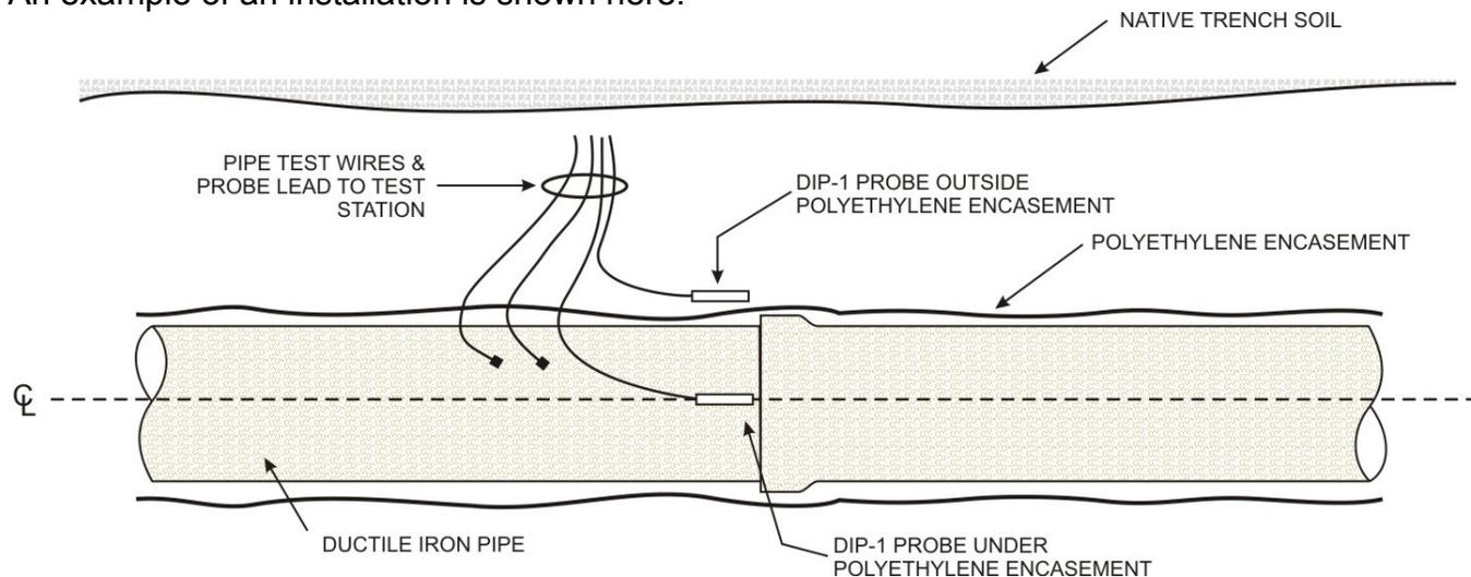
Note: The probes do not require that polyethylene encasement be used.
