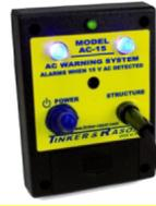
Super Bright Blue warning LEDs are visible in bright sunlight. Small Green LED shows unit in operation.
