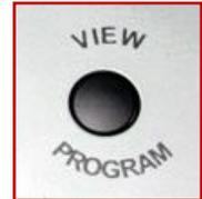
**NOTE:** When the Display is shown by pressing the View Program button, the instrument cannot be programmed. The Program button will not work until the Display is turned off by again pressing the View Program button, or by automatically shutting off. Once the Display is off, the Program button can be used.
