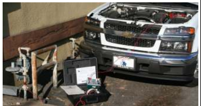
TYPICAL CONNECTION ACROSS INSULATED METER
